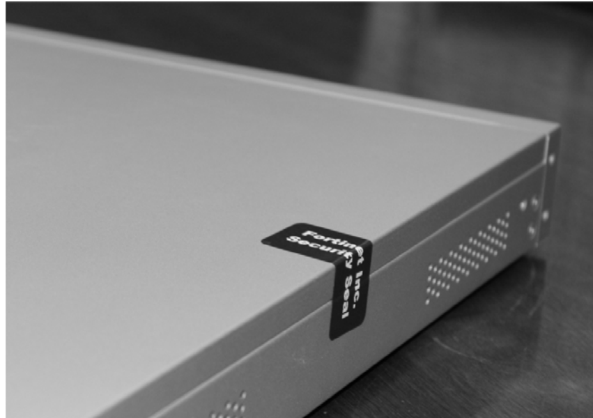
Figure 6: FortiGate-200A, 200A-HD, 300A, 300A-HD, 500A, 500A-HD and 800 tamper seal placement
