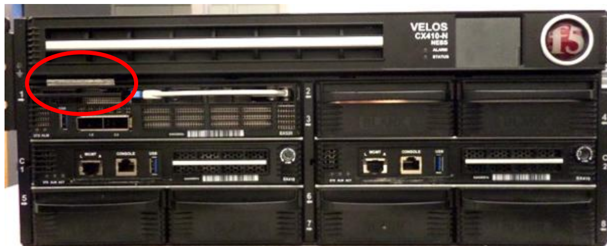
Figure 14 – Tamper labels on VELOS CX410-BX520 blade mounted on chassis (1 of 1 tamper label shown).
