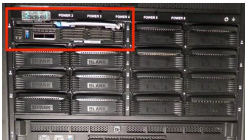
Figure 15 – Tamper labels VELOS CX1610-BX520 blade mounted on chassis (1 of 1 tamper label shown).
