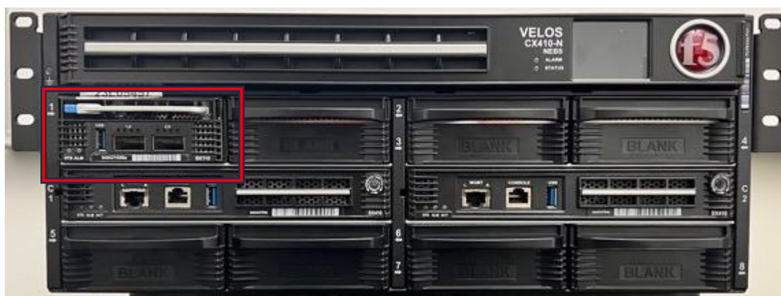
Figure 6 – VELOS CX410-BX110 with 7 filler panels and one blade. The tested blade VELOS CX410-BX110 in slot #1 delineated with red rectangle.
