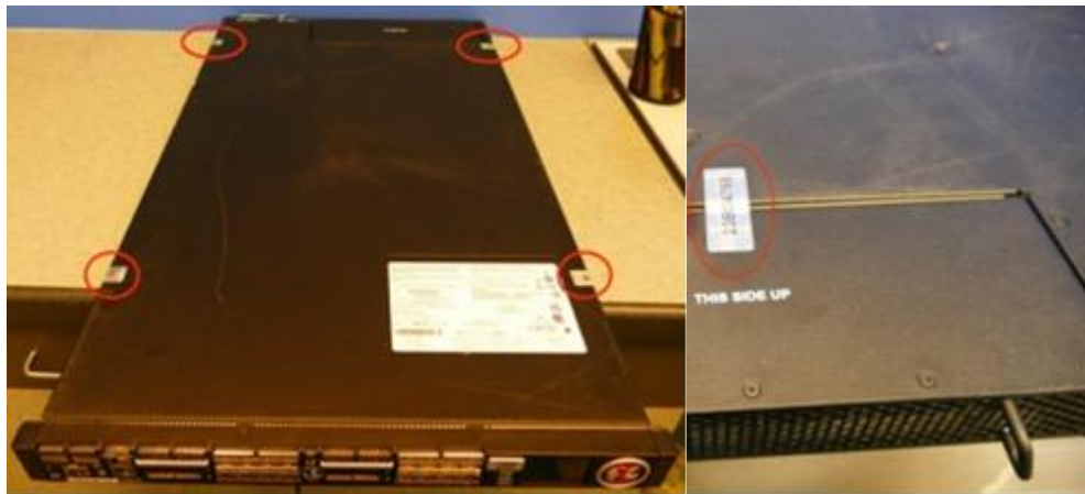
Figure 12 – Tamper labels on r10900, r10920-DF and r12900.
