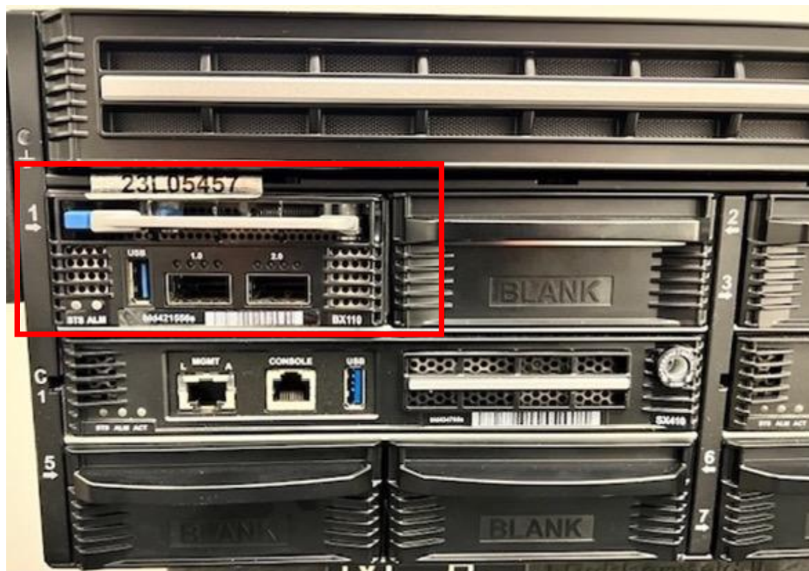
Figure 13 – Tamper labels on VELOS CX410-BX110 blade mounted on chassis.
