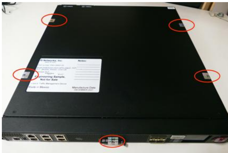
Figure 9 - Tamper labels on r4800 (5 of 5 tamper labels)
