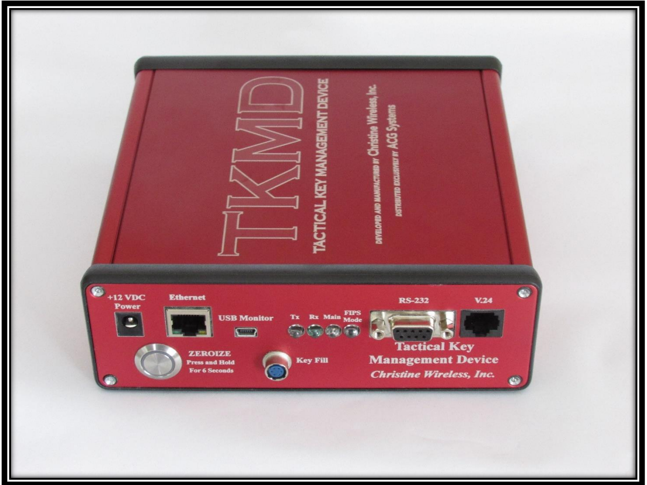
Figure 1: TKMD Top and Front View
