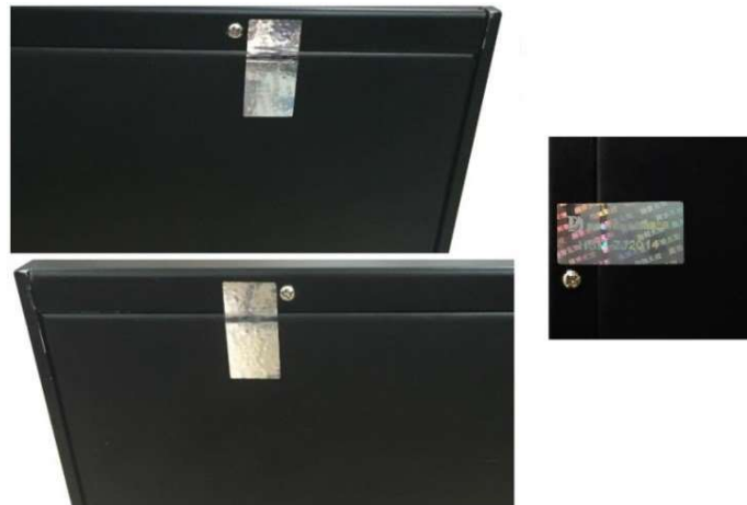
Figure 9: Tamper Evident Seals
