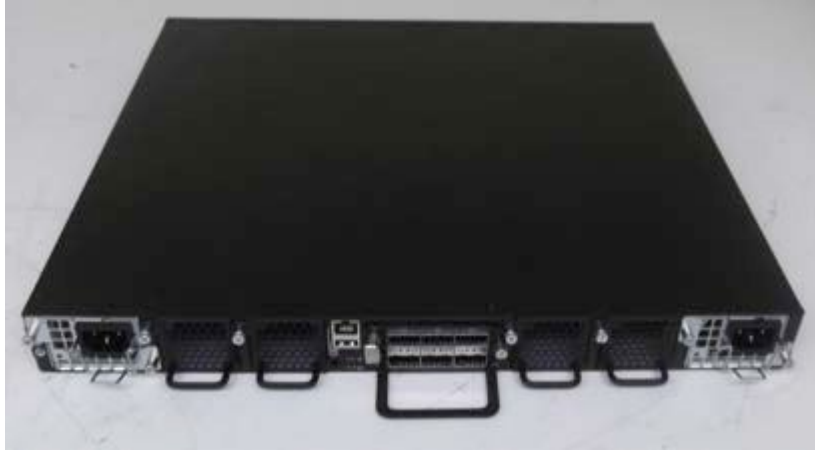
Figure 17 - Back Side of the ICX 7750-48F with Optional ICX7750-6Q Module
