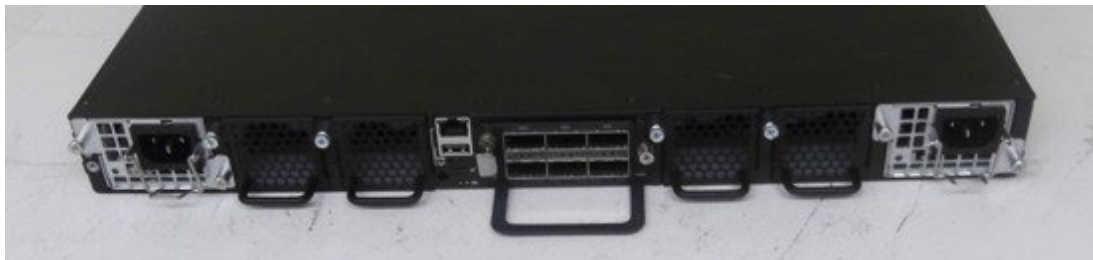
Figure 27 - Back Side of the ICX 7750-26Q with Optional ICX7750-6Q Module
