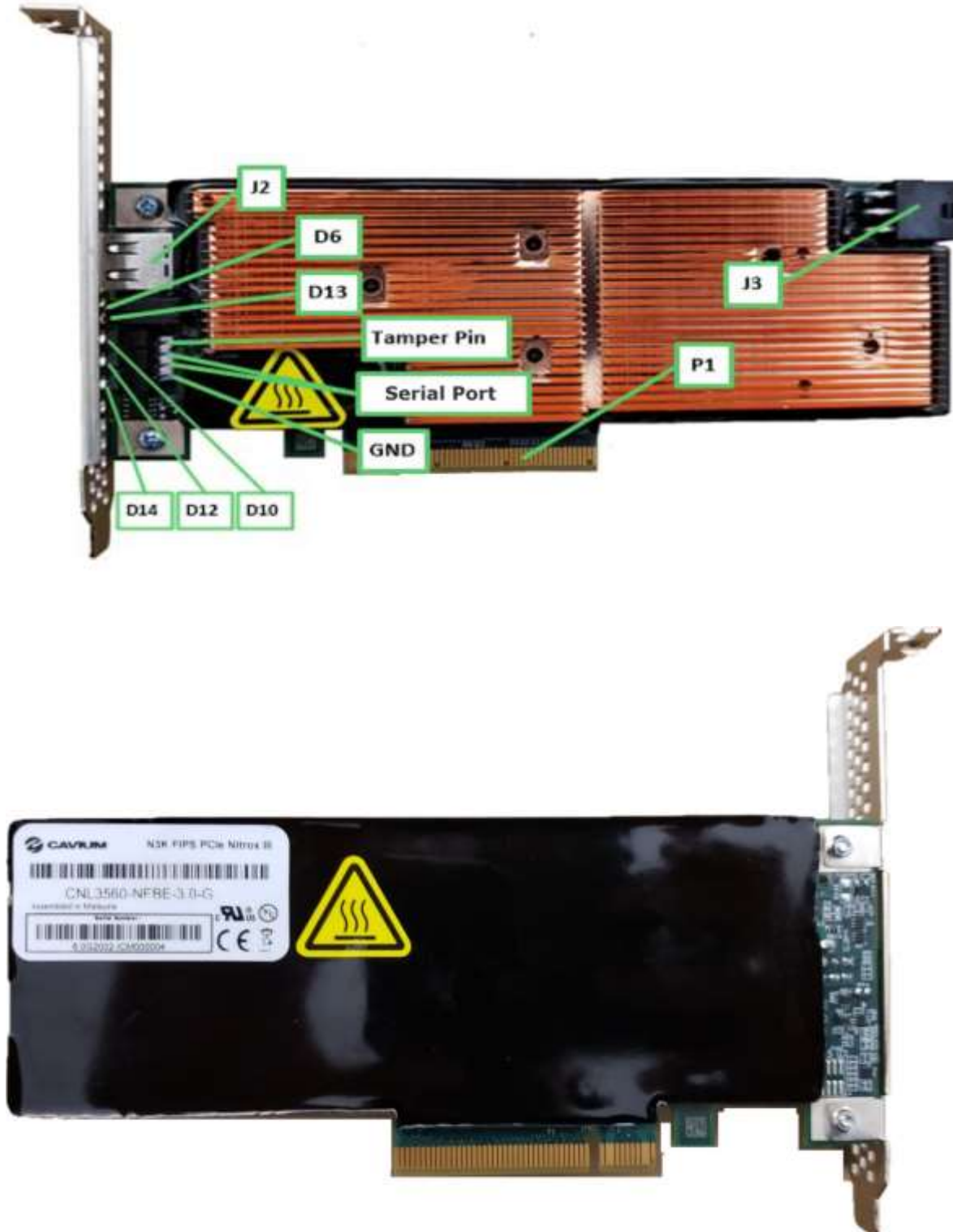
Figure 3 – Top View and Bottom View of Cryptographic Module (HW-3.0)
