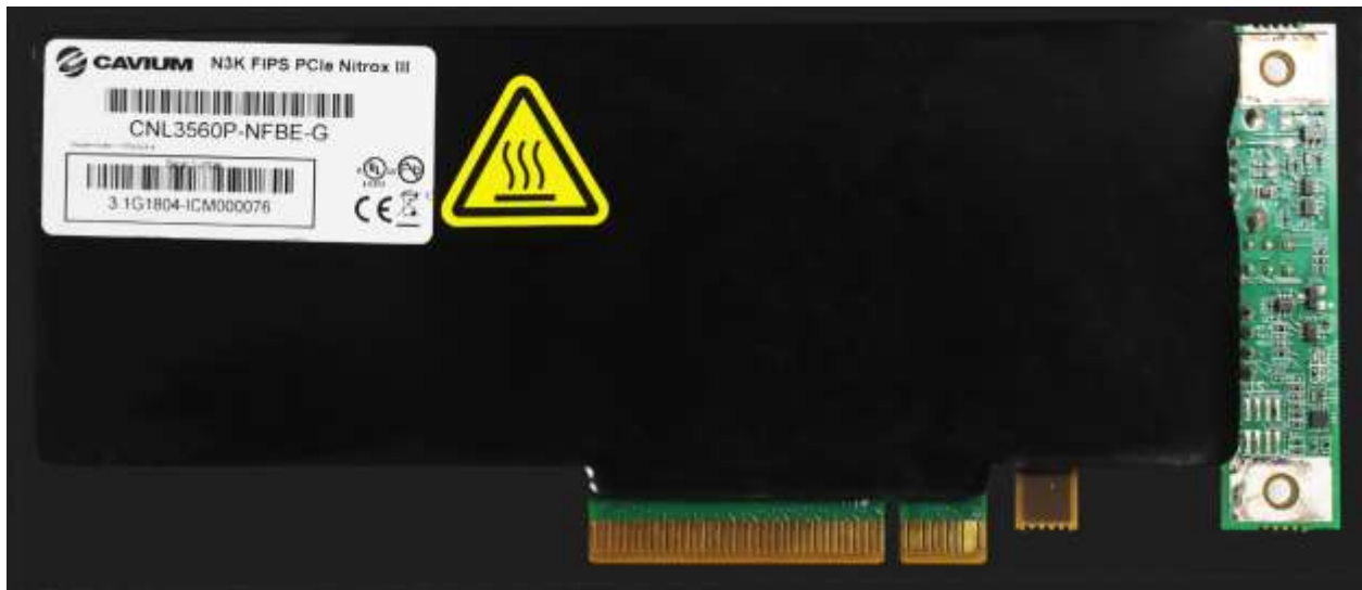
Figure 1 – Top View and Bottom View of Cryptographic Module (HW-1.0)
