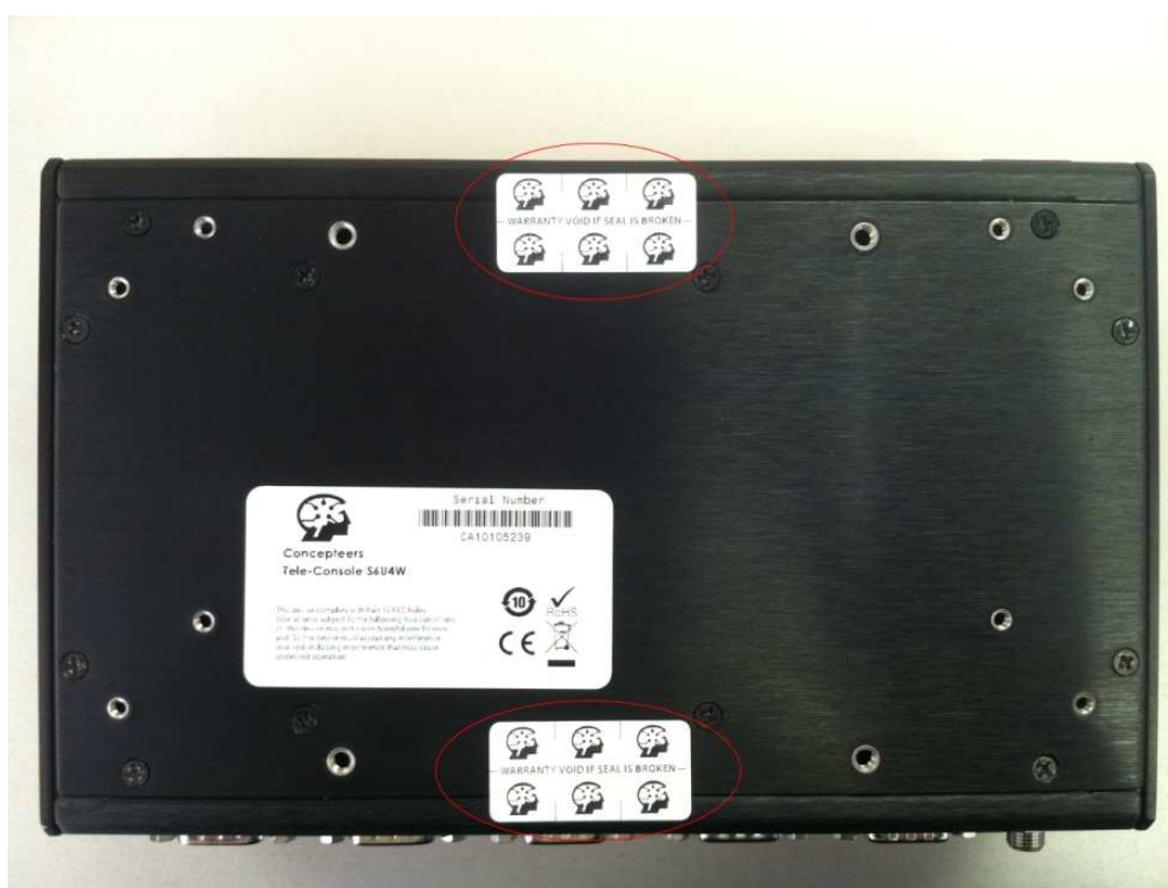
Figure 2 – Tamper Evidence Labels Placement (Bottom)
