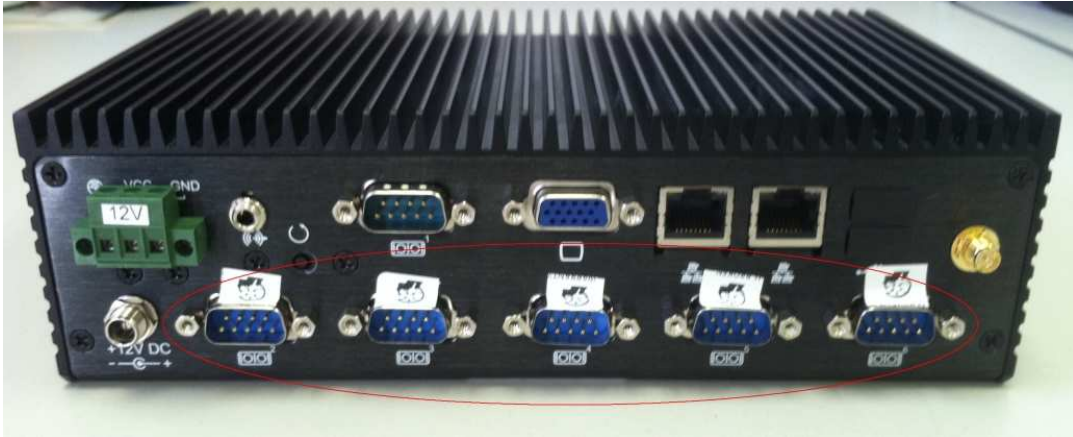
Figure 3 – Tamper Evidence Labels Placement (Rear)
