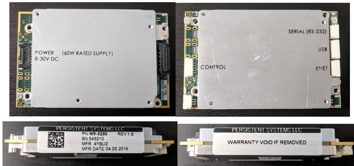
Figure 2 – Physical Boundary of Embedded Module Lite
