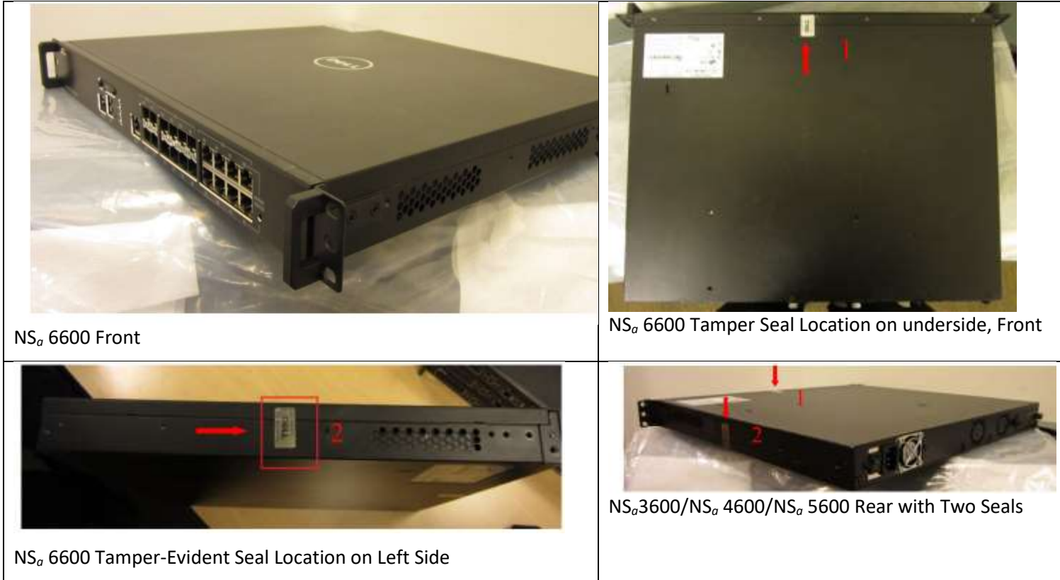
Figure 20: NS α 6600/NS α 5600/NS α 4600/NS α 3600 Front and Back Seals
