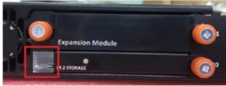
Figure 22: NS a 2650/NS a 3650/NS a 4650/NS a 5650 Tamper Evident Seal placement
