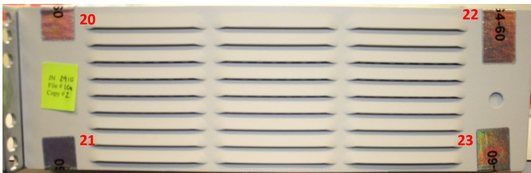
Figure 15 Location of Security Seals on Louver Panel (Right Side)
