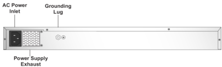
Figure 10 - PA-3020 / PA-3050 Back Interfaces
