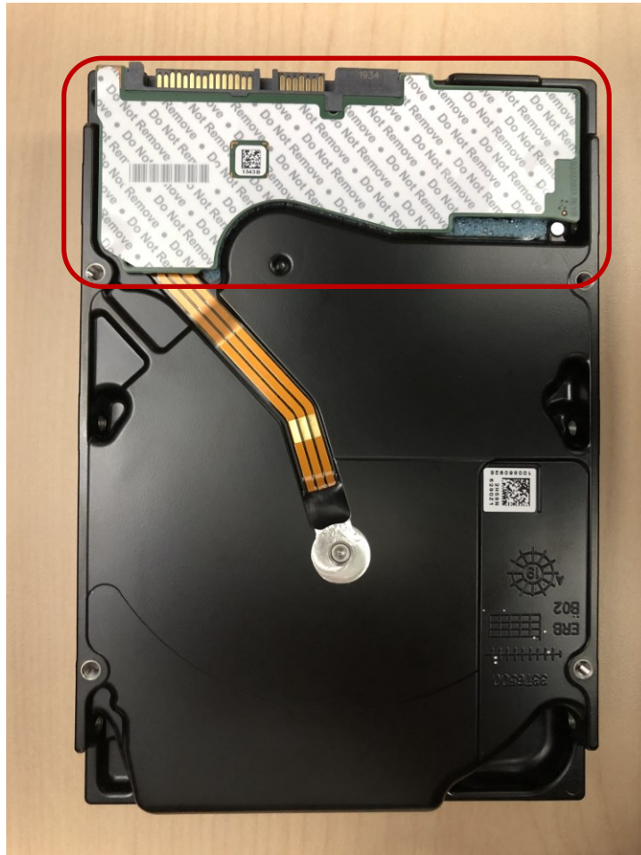
Figure 3: Module 1 Seal Application Locations
