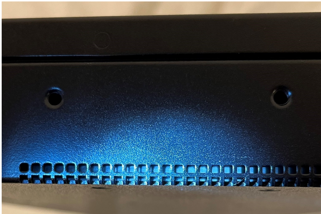
FIGURE 16: DEPICTION OF VENT PROTECTED BY INTERNAL BAFFLE
