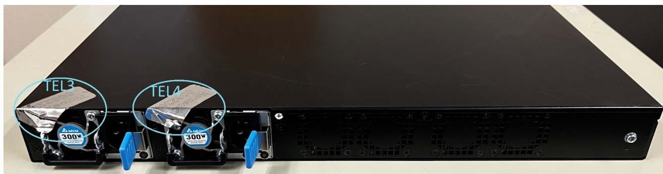
FIGURE 9: 2210 REAR TEL PLACEMENTS
