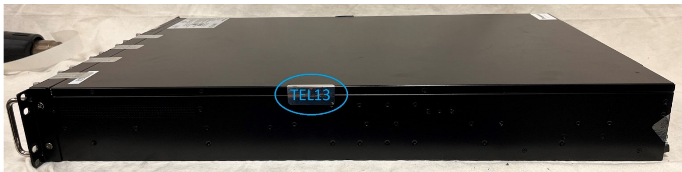
FIGURE 13: 3400 SERIES RIGHT SIDE TEL PLACEMENT
