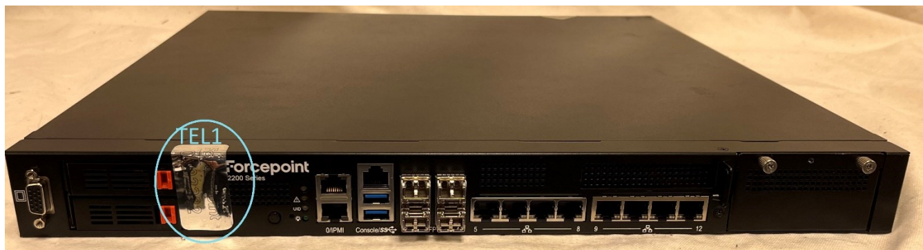
FIGURE 10: 2201 FRONT TEL PLACEMENT
