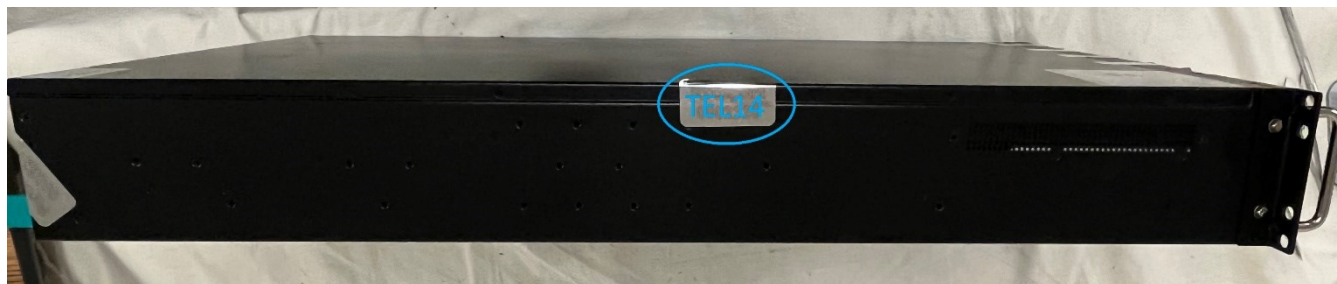
FIGURE 15: 3400 SERIES LEFT SIDE TEL PLACEMENT
