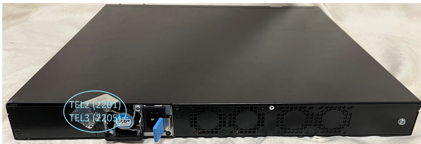
FIGURE 11: 2201/2205 REAR TEL PLACEMENT
