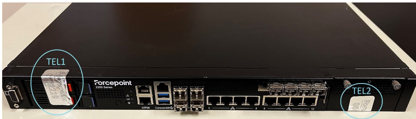
FIGURE 8: 2205/2210 FRONT TEL PLACEMENTS
