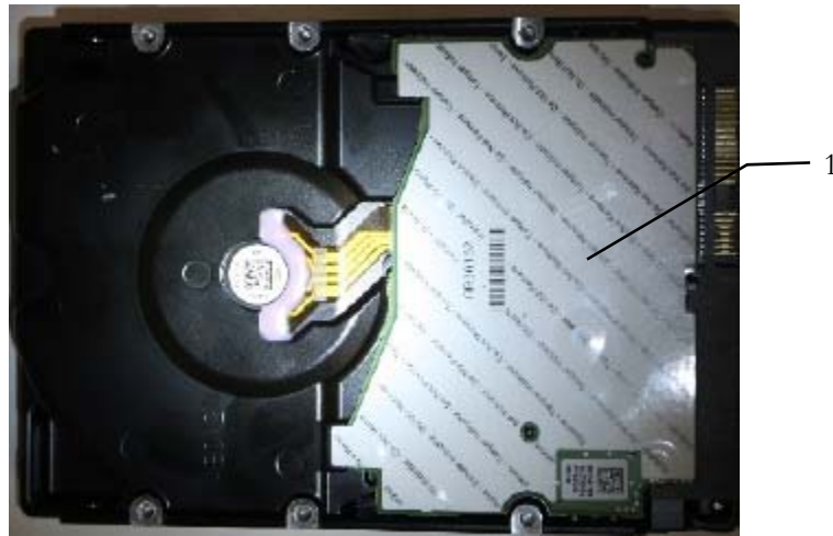
Figure 3: Tamper-Evident Seal over PCBA
