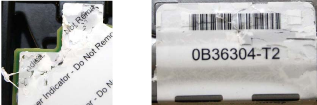
Figure 5: Tamper Evidence on Tamper Seals
