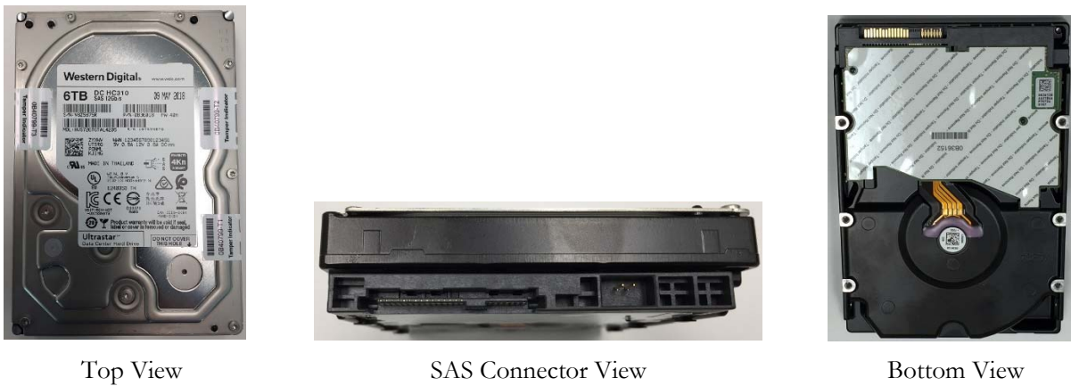
Figure 1: Ultrastar DC HC310 Cryptographic Boundary
