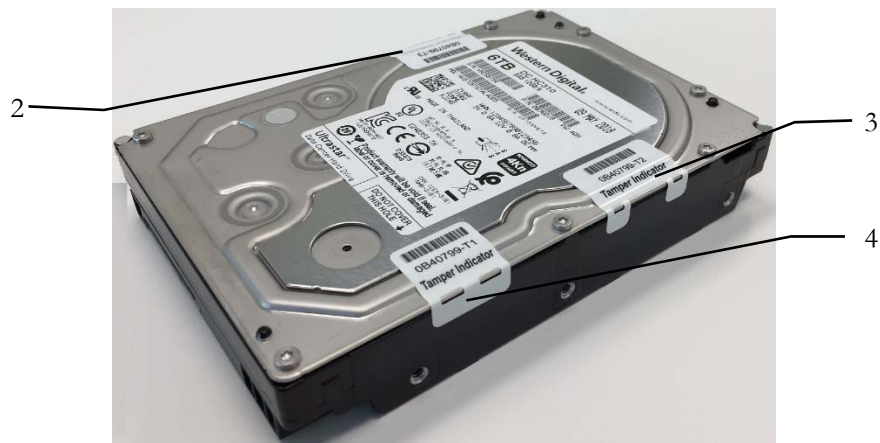
Figure 4: Wrapping Tamper-Evident Seals
