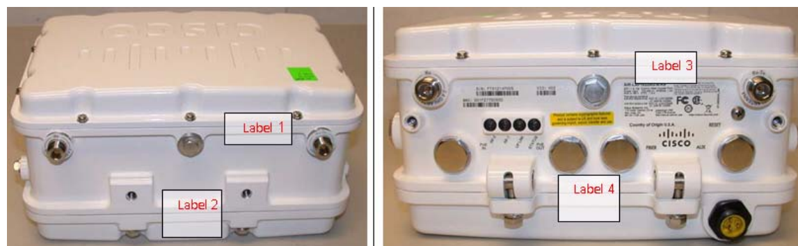
Figure 1 Tamper labels on AP1522, AP1524PS, and AP1524SB
