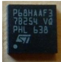
Figure 4: Picture of the Cryptographic Module (VQFN32) – Marking
