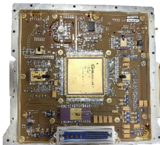
Figure 2. TASE-CM-VIPER Hardware Cryptographic Module
