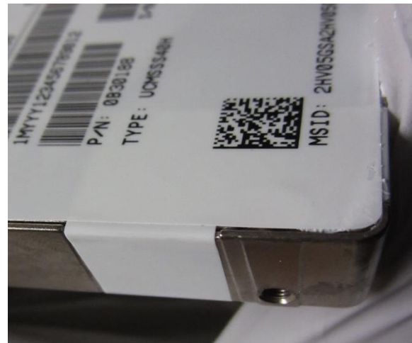
Figure 5 - Smaller Tamper-Evident Label Underneath Large Label Wrapping Down Sides, Hardware Revision (0001) only
