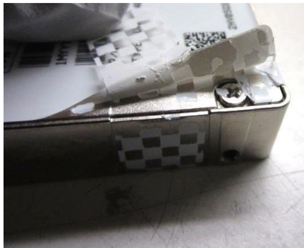
Figure 7 - Tamper Evidence on Smaller Tamper-Evident Label, Hardware Revision (0001) only
