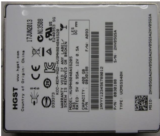
Figure 4 - Large Tamper-Evident Label on Top Surface
