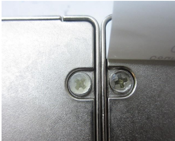
Figure 9 - Left side shows tamper. Right side shows no tamper.
