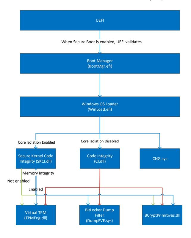
Boot Manager checks the integrity of the WINLOAD.EFI component of the Windows OS Loader before it is loaded.
