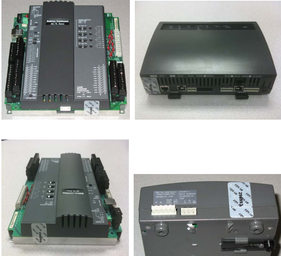
Figure 3 depicts the ACX Series Rev 2a Controller (left) with a tamper evident seal on the top of the enclosure and a second tamper evident seal on the bottom of the enclosure. Figure 3 also depicts The NetController II Rev B Controller (right) with a tamper evident seal on the left side of the enclosure and a second tamper evident seal on the bottom of the enclosure.
