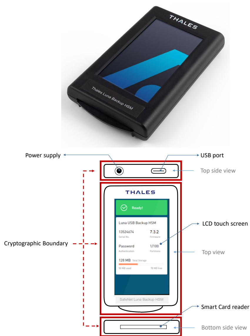
Figure 1: Thales Luna Backup HSM Cryptographic Module and cryptographic boundary
