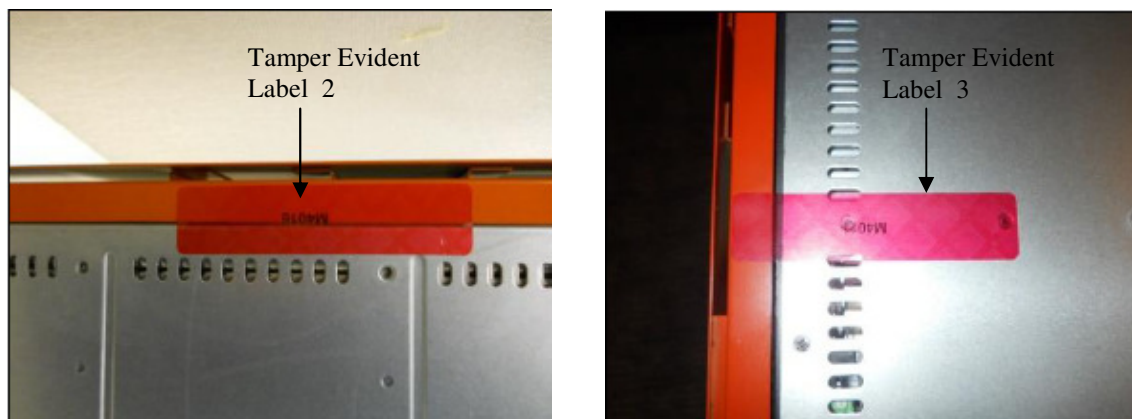
Figure 6 – Sealed front bezel to chassis bottom (Left) and Sealed front bezel to chassis top (Right)
