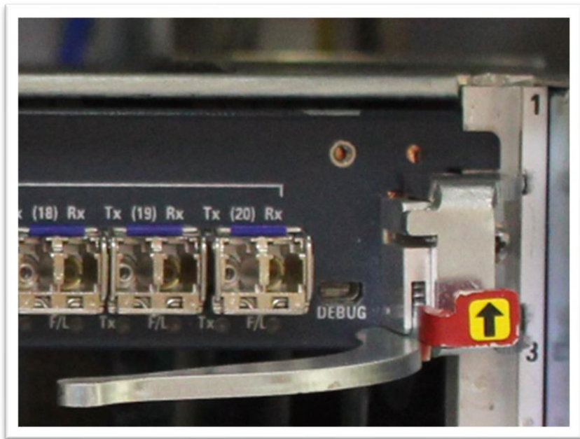
Figure 9: Front Panel Before Installing Pick Resistant Lock
