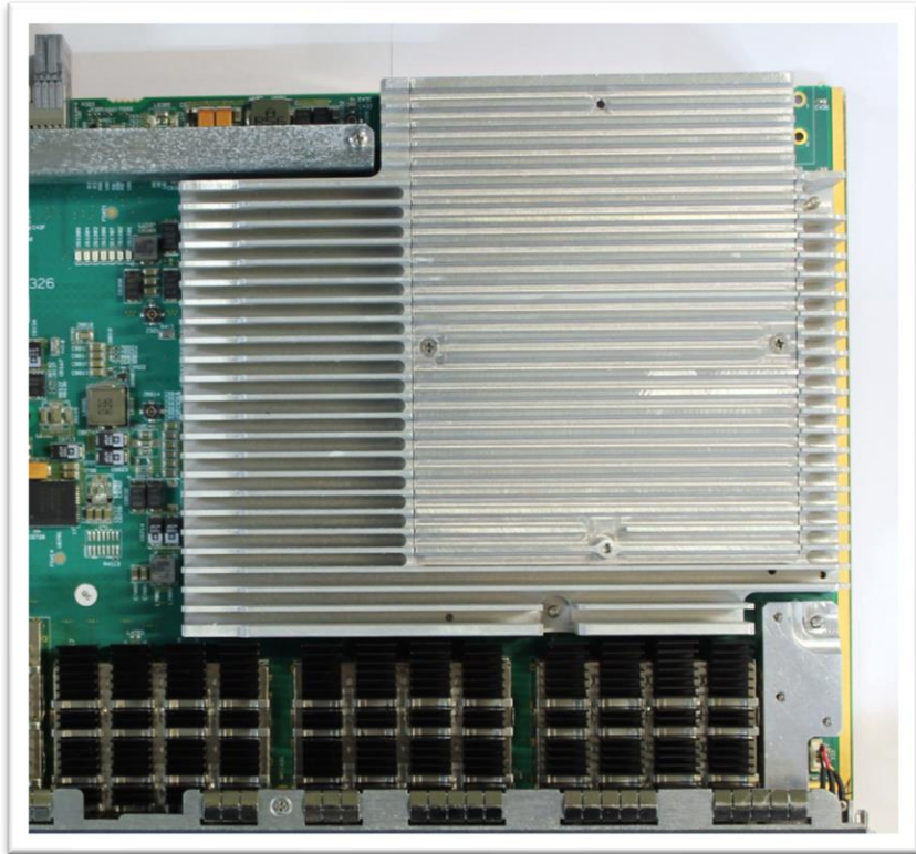
Figure 8: Metallic Tamper Shield Sealed and Mated with the PCB (front)
