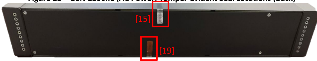
Figure 28 – OSN 1800IIE (AC Power) Tamper-Evident Seal Locations (Back)
