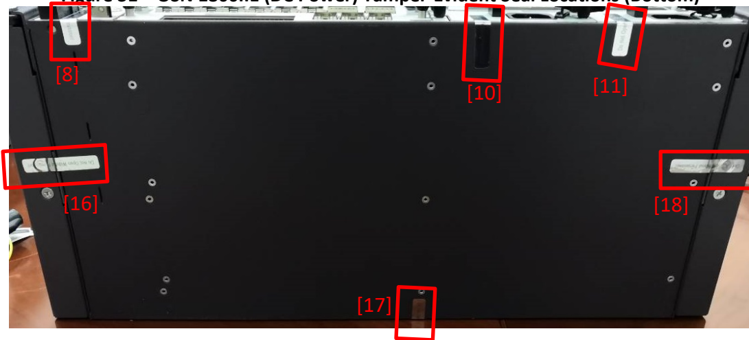
Figure 31 – OSN 1800IIE (DC Power) Tamper-Evident Seal Locations (Bottom)
