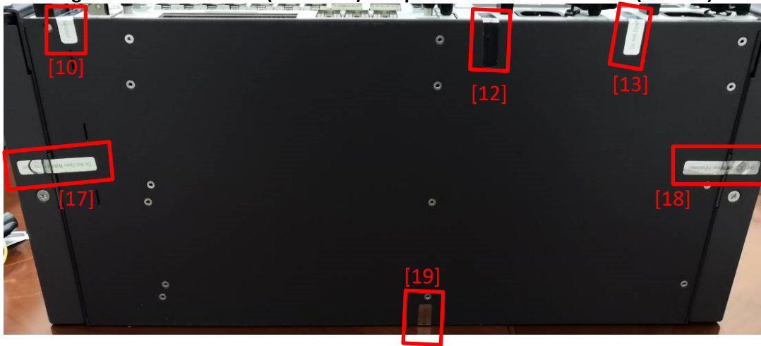
Figure 27 – OSN 1800IIE (AC Power) Tamper-Evident Seal Locations (Bottom)
