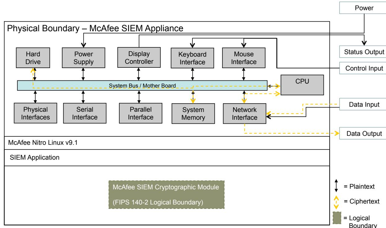
**Figure 1 – Module Boundary and Interfaces Diagram**
