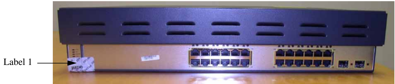
Figure 3 Placement of Tamper evident label on the cap of the mode button
