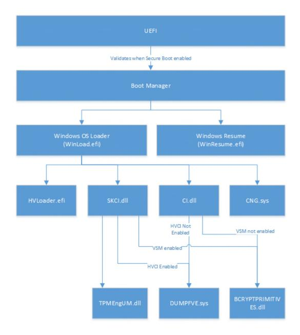
The following diagram describes the Integrity Chain of trust for each supported configuration for the following versions:
