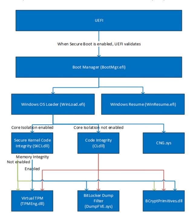
The integrity of the BitLocker Dump Filter module is checked according to the following:
