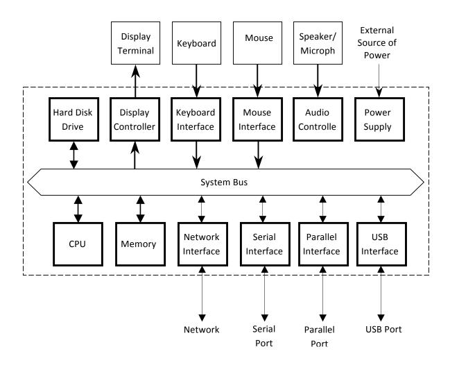
Figure 1: Cryptographic Module Hardware Block Diagram
