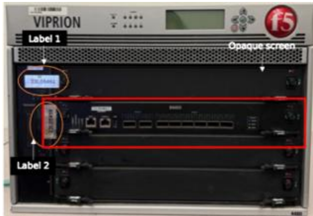
Figure 7 – Tamper labels on chassis with VIPRION B4450 blade (delineated by a red box) and three blanks (2 of 2 tamper labels shown)
