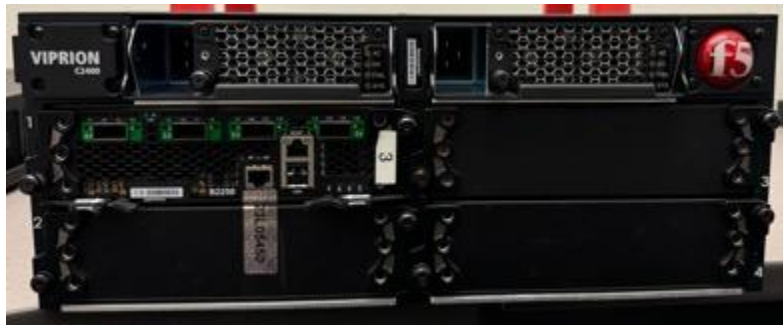
Figure 3 - B2250 blade mounted in VIPRION chassis C2400
