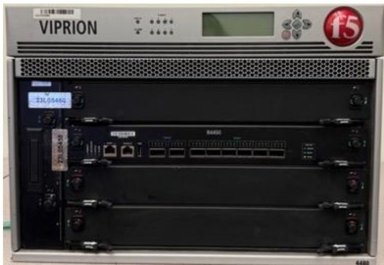
Figure 4 - B4450 blade mounted in VIPRION chassis C4480
