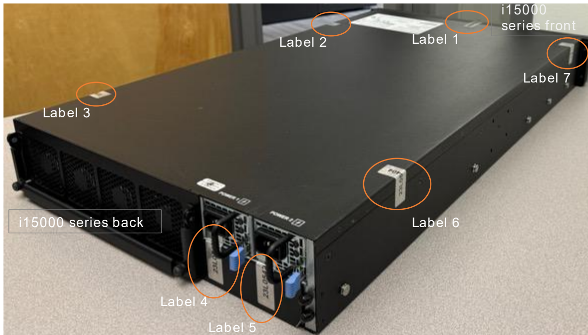
Figure 5 – Tamper labels on BIG-IP i15600, BIG-IP i15800, and BIG-IP i15820-DF.
