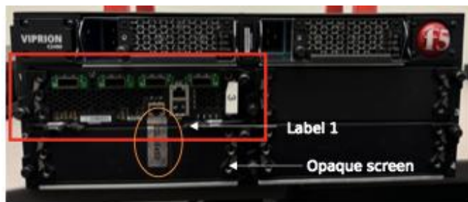
Figure 6 – Tamper labels on chassis with VIPRION B2250 blade (delineated by a red box) and three blanks (1 of 1 tamper label shown)
