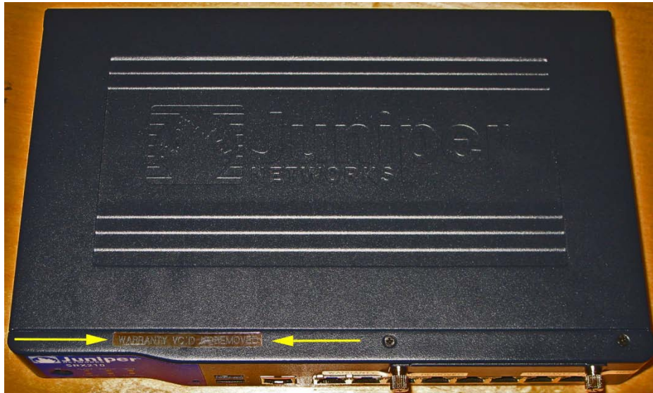
Figure 3. SRX210 Tamper Evident Seal Location (Top)
