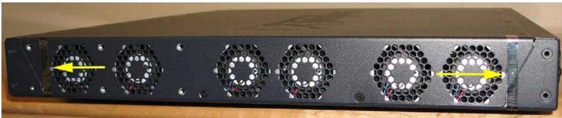
Figure 8. SRX240 Tamper Evident Seal Location (Left Side)
