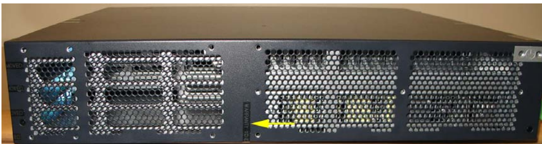
Figure 11. SRX650 Tamper Evident Seal Location (Right Side)
