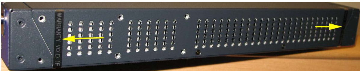
Figure 7. SRX240 Tamper Evident Seal Location (Right Side)
