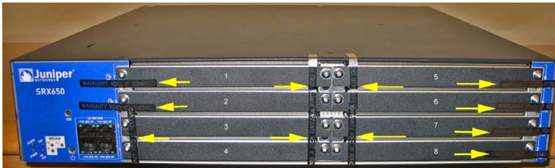
Figure 9. SRX650 Tamper Evident Seal Locations (Front)
