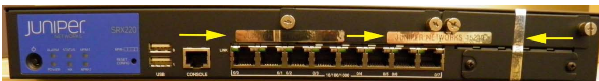
Figure 4. SRX220 Tamper Evident Seal Location (Front)
