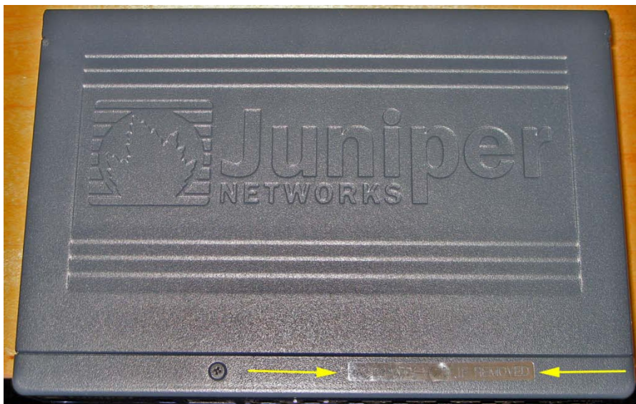
Figure 2. SRX100 Tamper Evident Seal Location (Top)
