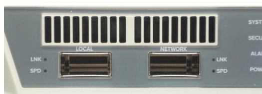
Figure 11 – A9100B 100G Ethernet ports close-up - CFP4s not installed
