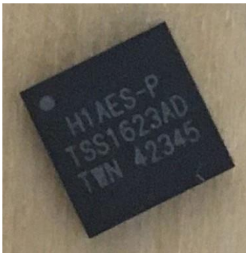
Figure 1 - Titan Security Key, Chip Boundary (Front)
