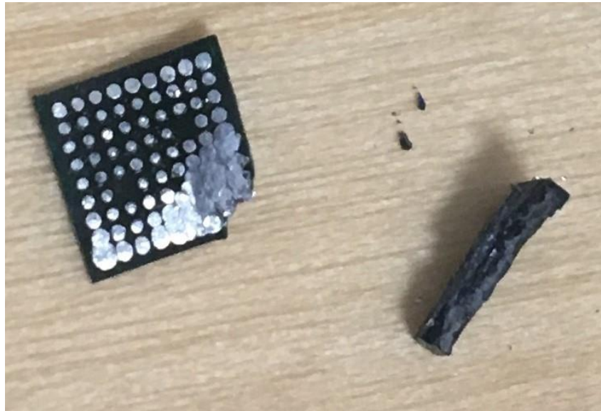
Figure 4- Tamper Evidence and damage to the module
