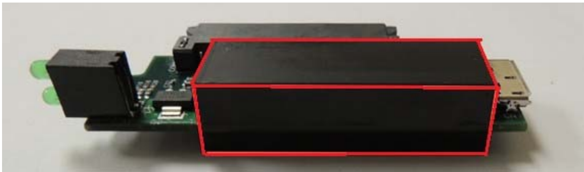
Figure 3 – KDH350-CM –Right side view. The cryptographic boundary is defined by the area that the epoxy potting covers, which is outlined in red.
