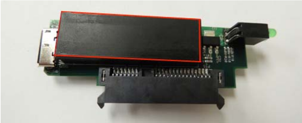
Figure 1 – KDH350-CM – Top side view. The cryptographic boundary is defined by the area that the epoxy potting covers, which is highlighted in red.
