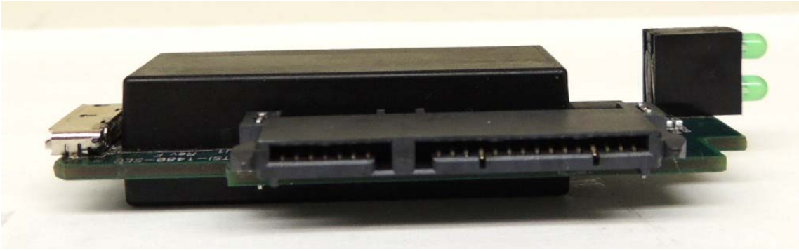
Figure 6 – KDH350-CM – Left side view demonstrating the SATA port.
