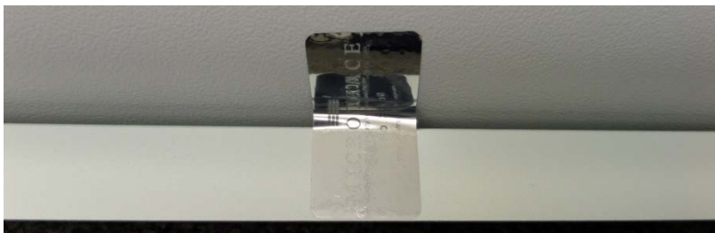
Tamper seal applied over small gap between metal backing and plastic cover
