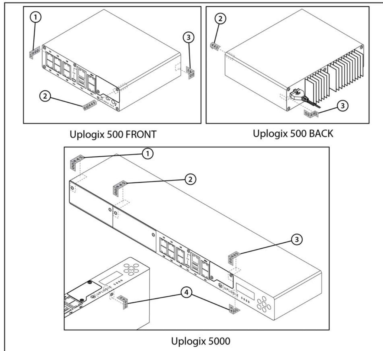
Figure 10: Tamper Label Placement on the 500 and 5000
