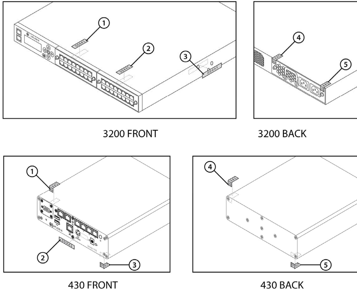
Figure 9: Tamper Label Placement on the 430 and 3200
