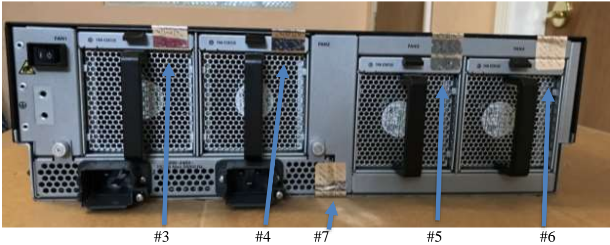
Figure 10: FPR9300 Series Rear view (Rear has TEL #3, #4, #5, #6, each overlapping chassis and plug-in and #7 on bottom)
