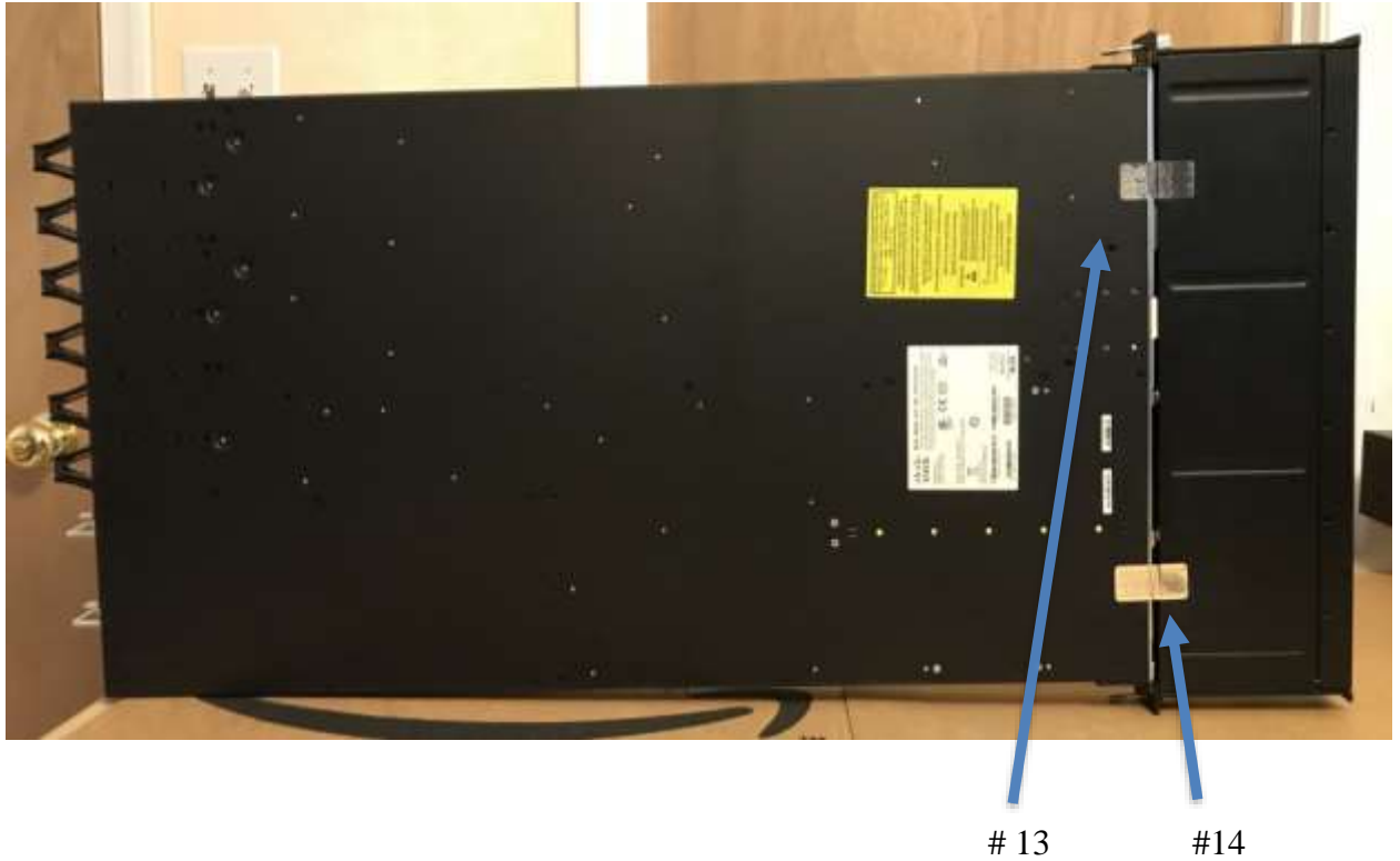
Figure 6: FPR4100 Series Bottom view (Bottom shows TEL #13 and #14 overlapping opacity shield and 4000 chassis)
