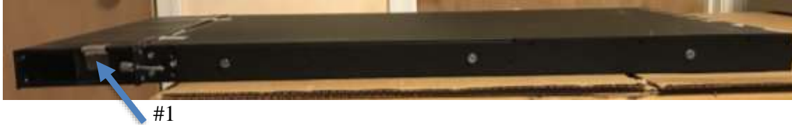
Figure 2: FPR4100 Series Right Side (Right side has TEL #1 overlapping top and side)
