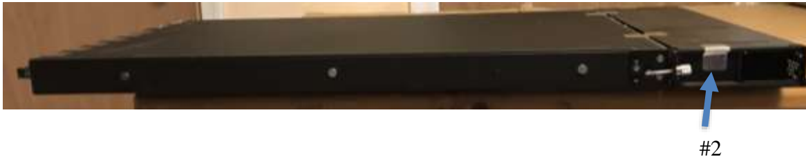
Figure 3: FPR4100 Series Left Side (Left side has TEL #2 overlapping top and side)
