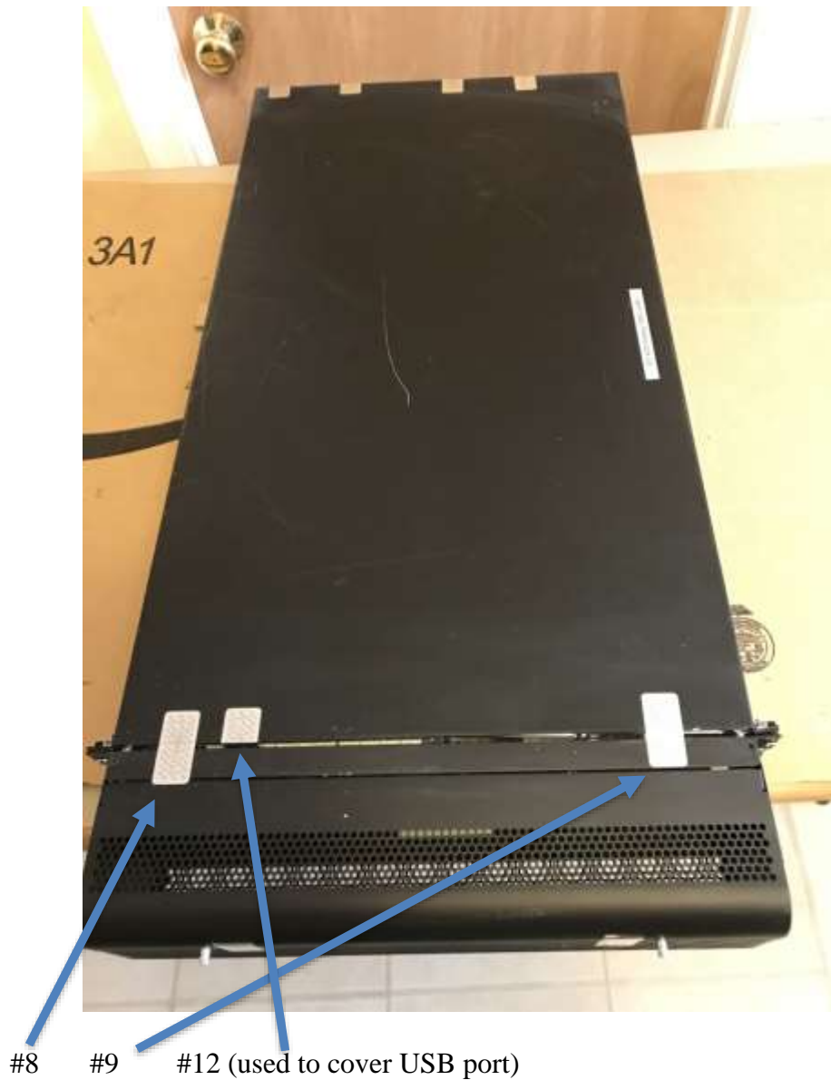
Figure 11: FPR9300 Series Top view (Top has TEL #8 and #9 overlapping opacity shield and top of chassis, also present is TEL #3, #4, #5 and #6 listed on Back view. TEL #12 partially obscured inside the opacity shield, overlapping front of chassis and top of chassis covering the USB)
