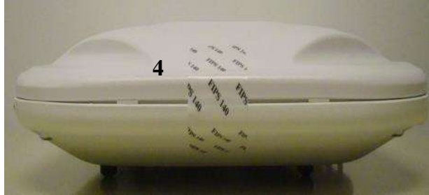
Figure 36 Cisco Aironet 1602i Tamper Evident Label Placement (Front, Back, Top, Bottom, Left, Right)
