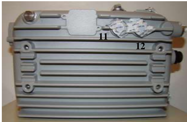
Figure 35 Cisco Aironet 1572 Tamper Evident Label Placement (Front, Back, Top, Bottom, Left, Right)
