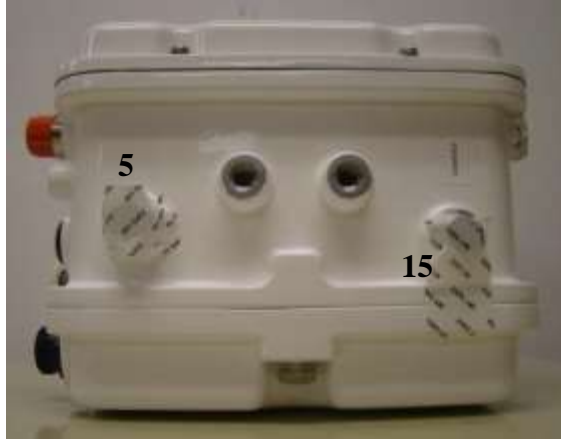
Figure 33 Cisco Aironet 1552e Tamper Evident Label Placement (Front, Back, Top, Bottom, Left, Right)
