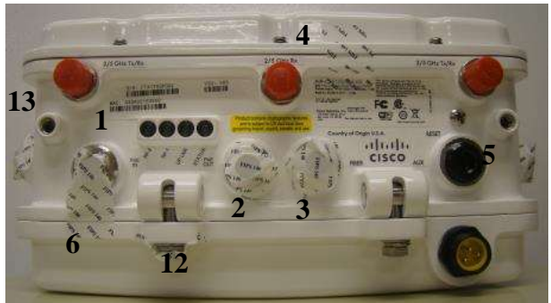
Figure 32 Cisco Aironet 1532i Tamper Evident Label Placement (Front, Back, Top, Bottom, Left, Right)
