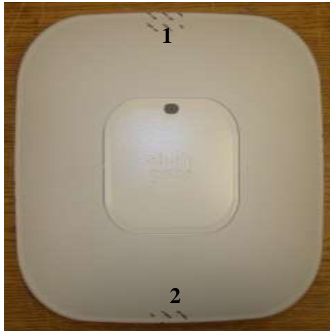
Figure 45 Cisco Aironet 3602e/p Tamper Evident Label Placement (Top, Bottom, Front, Back, Left, Right)
