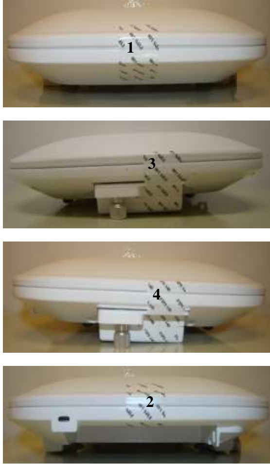
Figure 46 Cisco Aironet 3602i Tamper Evident Label Placement (Top, Bottom, Front, Back, Left, Right)
