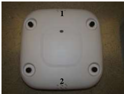
Figure 40 Cisco Aironet 2602i Tamper Evident Label Placement (Top, Bottom, Front, Back, Left, Right)
