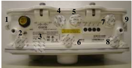
Figure 33 Cisco Aironet 1552e Tamper Evident Label Placement (Front, Back, Top, Bottom, Left, Right)
