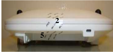
Figure 45 Cisco Aironet 3602e/p Tamper Evident Label Placement (Top, Bottom, Front, Back, Left, Right)
