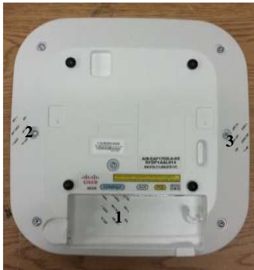
Figure 38 Cisco Aironet 1702 Tamper Evident Label Placement (Front, Back, Top, Bottom, Left, Right)
