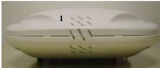
Figure 35 Cisco Aironet 1572 Tamper Evident Label Placement (Front, Back, Top, Bottom, Left, Right)
