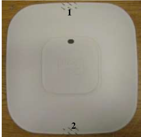
Figure 39 Cisco Aironet 2602e Tamper Evident Label Placement (Top, Bottom, Front, Back, Left, Right)
