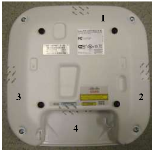
Figure 37 Cisco Aironet 1602e Tamper Evident Label Placement (Front, Back, Top, Bottom, Left, Right)
