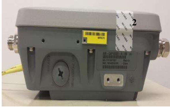
Figure 31 Cisco Aironet 1532e Tamper Evident Label Placement (Front, Back, Bottom, Top, Left, Right)
