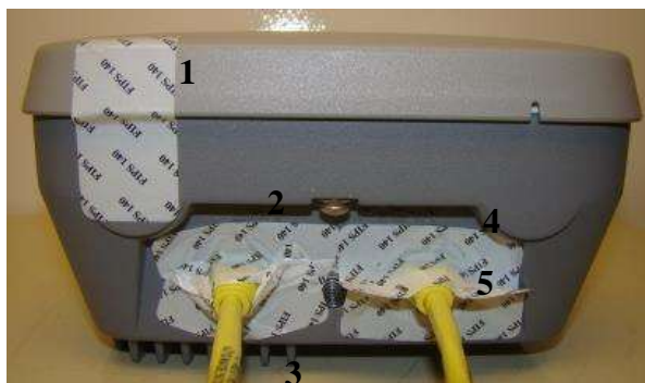
Figure 31 Cisco Aironet 1532e Tamper Evident Label Placement (Front, Back, Bottom, Top, Left, Right)
