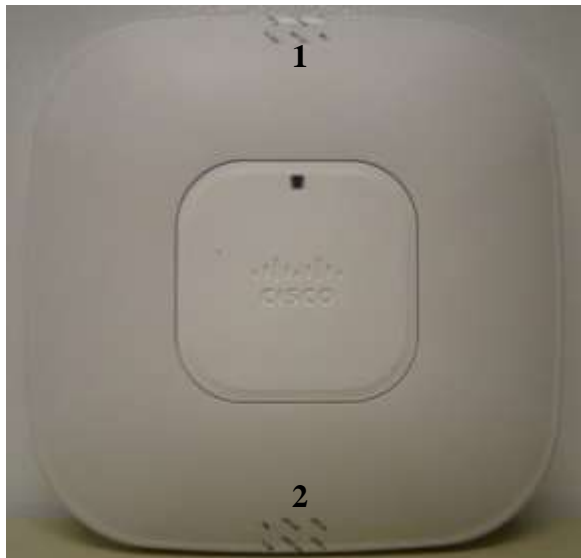
Figure 43 Cisco Aironet 3502e Tamper Evident Label Placement (Top, Bottom, Front, Back, Left, Right)
