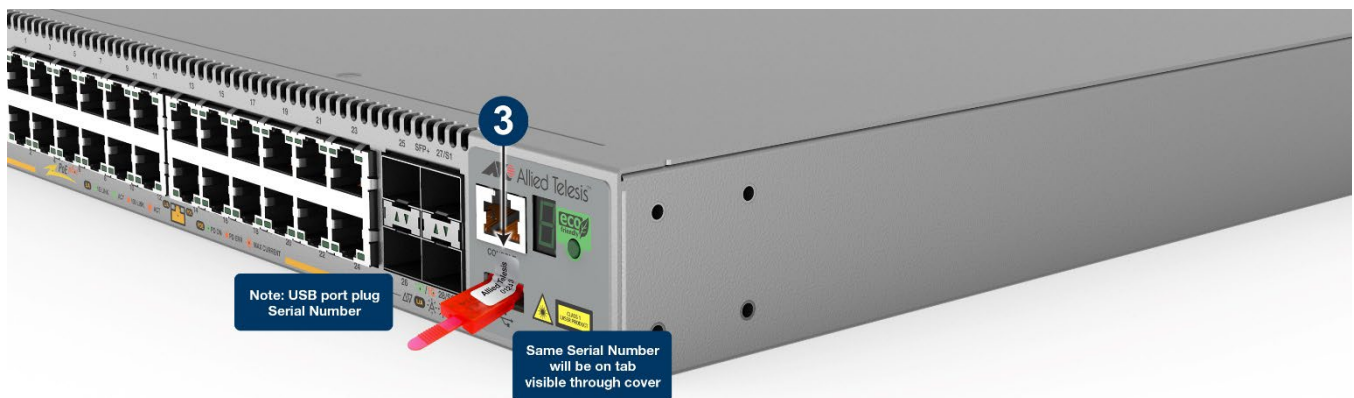
Figure 83: Location of USB Port Plug for x530L-28GPX
