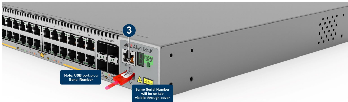
Figure 81: Location of USB Port Plug for x530L-28GTX
