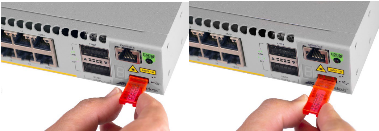
Figure 89: Removing the Housing from USB Port Lock
