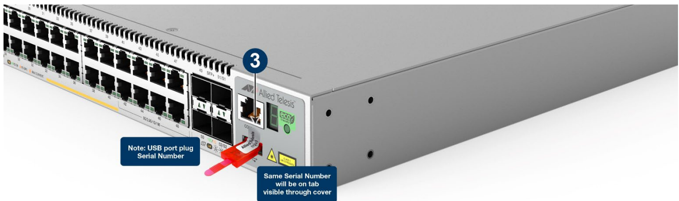
Figure 71: Location of USB Port Plug for x530-52GPXm
