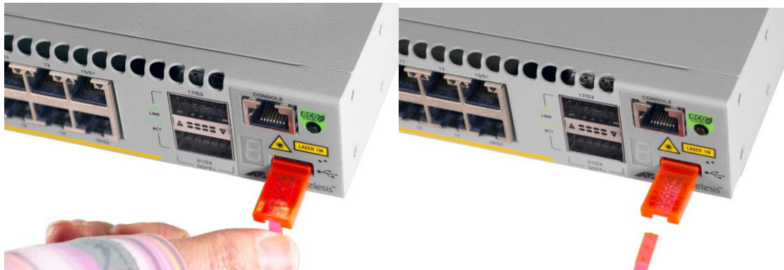
Figure 88: Breaking the Tab on USB Port Lock
