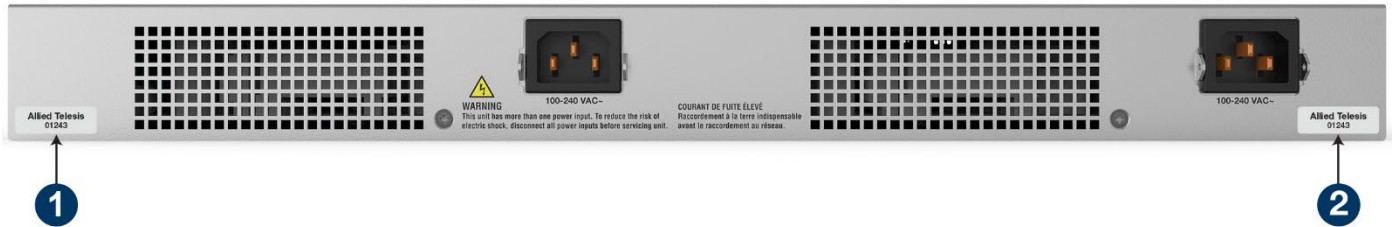
Figure 70: Tamper-Evident Seals on Rear of x530-52GPXm
