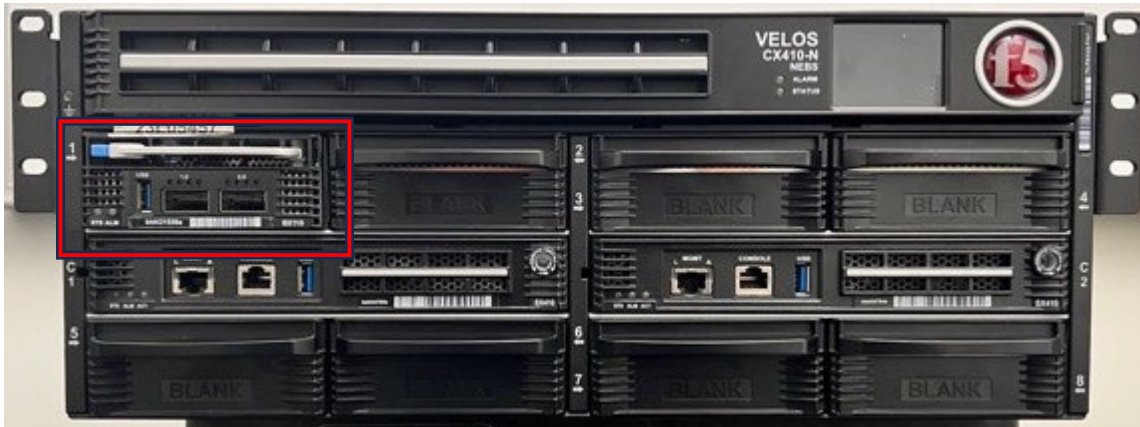
Figure 6 – VELOS CX410-BX110 with 7 filler panels and one blade. The tested blade VELOS CX410-BX110 in slot #1 delineated with red rectangle.
