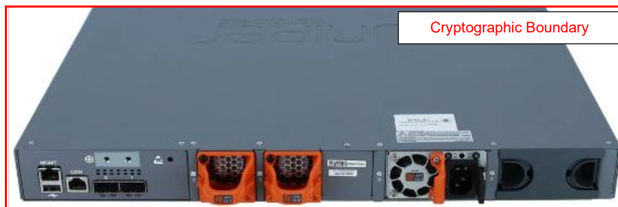
Figure 10 – Rear Panel EX3400-48P/48T
