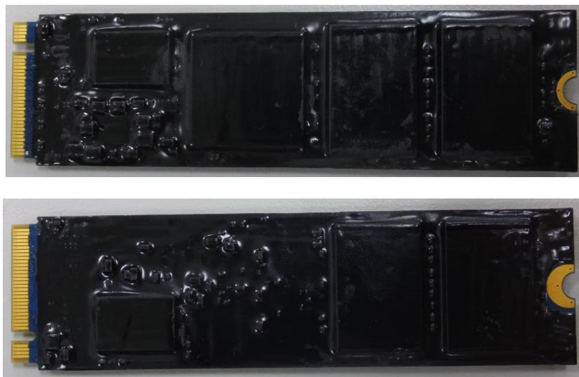
Exhibit 6 - Specification of the PS5012-E12 M.2 2280 NVMe NAND FLASH SSD Series Cryptographic Boundary (From top to bottom: top side, bottom side).
