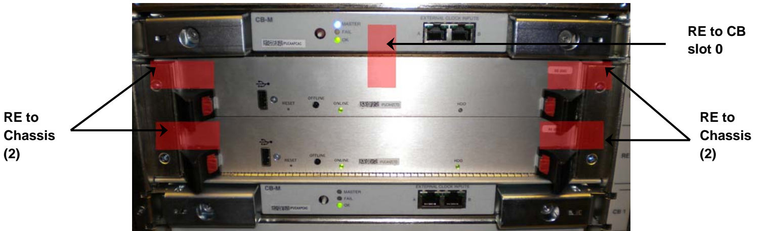
Figure 5. M320 with Routing Engine Tamper Label Placement (5 Tamper Labels)
