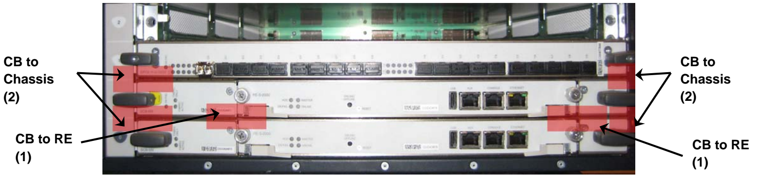
Figure 6. MX240, MX480, and MX960 with Routing Engine Tamper Label Placement (6 Tamper Labels)
