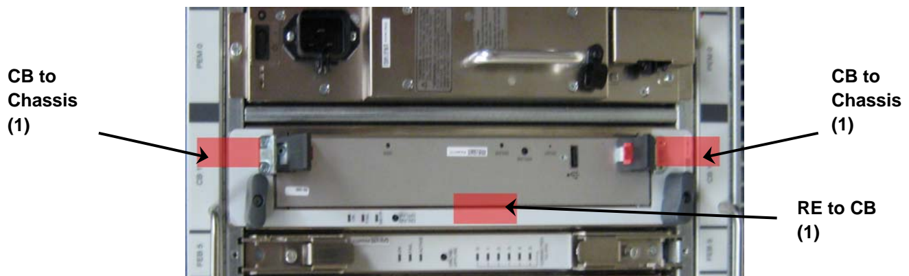
Figure 4. M120 with Routing Engine Tamper Label Placement (3 Tamper Labels)
