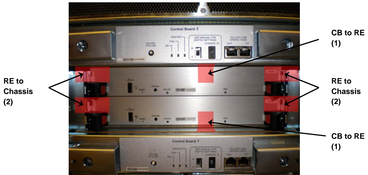
Figure 7. T320, T640, and T1600 with Routing Engine Tamper Label Placement (6 Tamper Labels)
