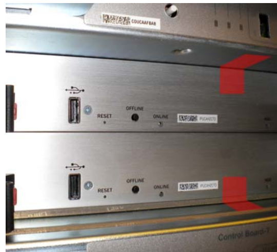
Figure 8. Alternate View - T320, T640, and T1600 with Routing Engine Tamper Label Corner Placement for CB to RE
