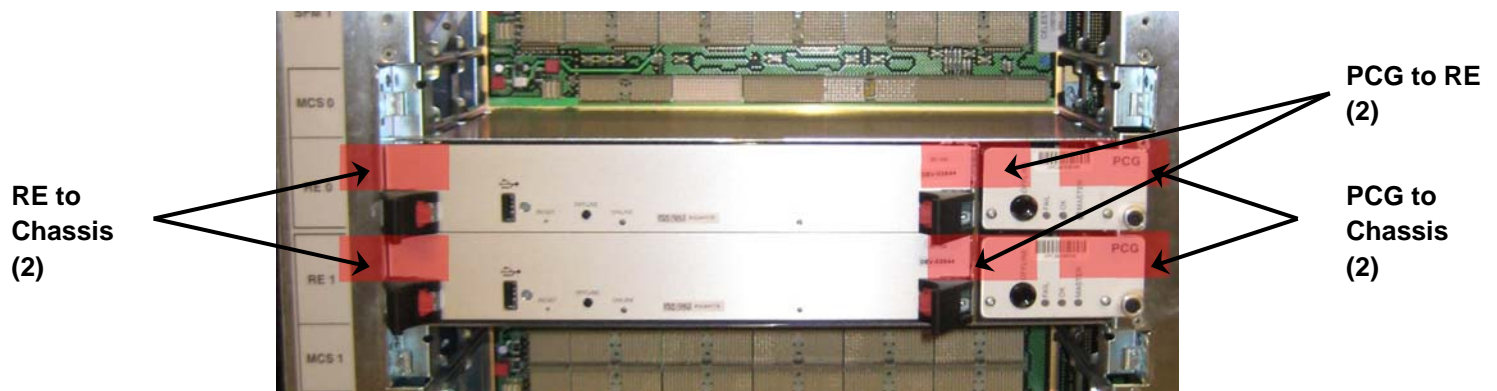
Figure 3. M40e with Routing Engine Tamper Label Placement (6 Tamper Labels)
