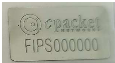
Figure 5 – cVu 16100 Tamper-Evident Seal
