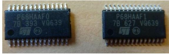
Figure 2: Picture of the Cryptographic Module (VQFN32) – Marking P68HAAF0 / P68HAAF1
