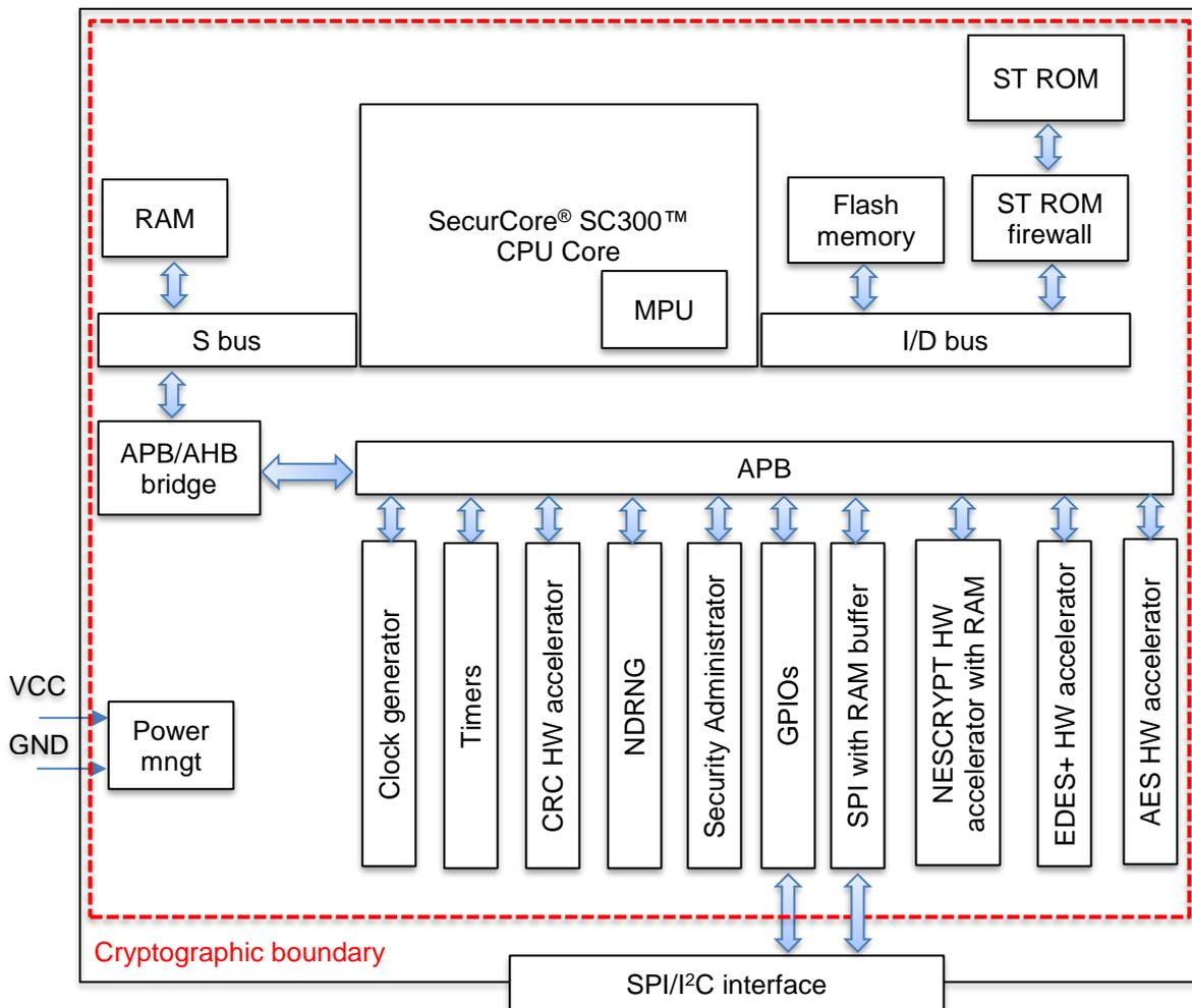
A block diagram of the TPM FW is provided in Figure 16: TPM FW block diagram.
