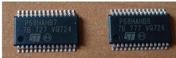
**Figure 6: Picture of the Cryptographic Module (VQFN32) – Marking P68HAHB7 & P68HAHB8**
