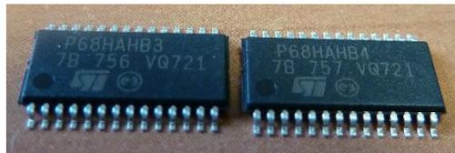
Figure 4: Picture of the Cryptographic Module (VQFN32) – Marking P68HAHB3 & P68HAHB4
