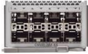
(a) 8-port 1/10 Gigabit Ethernet with SFP/SFP+
