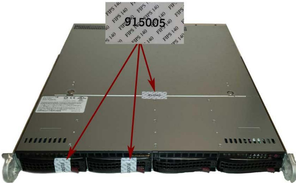
Figure 2 – Location of Tamper-Evident Seals
