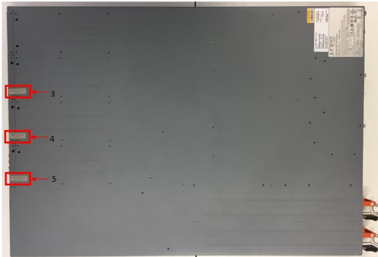
Figure 14 - SRX4100 & SRX4200 Bottom View: TEL 3, 4, 5
