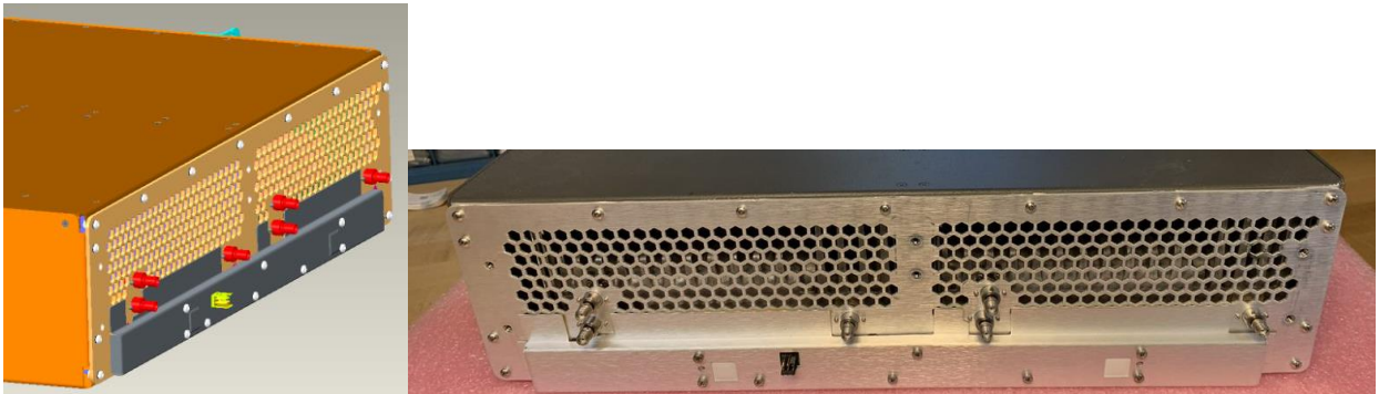
Figure 15: Cover on the rear side of the chassis for opacity of the digital board and protection of the back panel board
