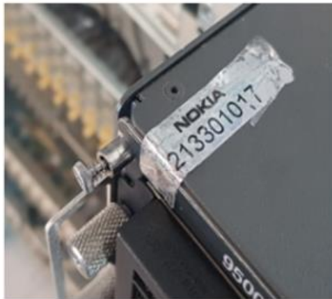
Figure 12: Tamper-evident label: broken (normal view)
