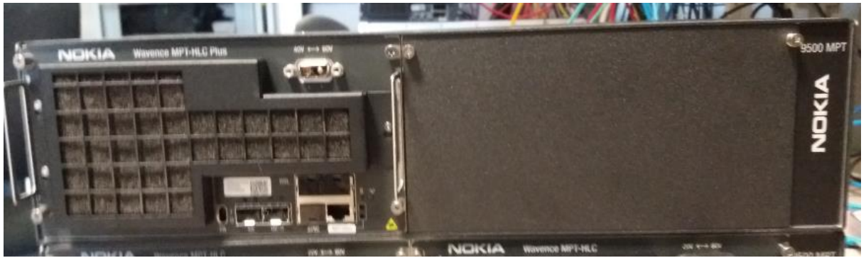
Figure 3: Front of the chassis with one MPT-HLC module inserted while the other slot is covered with a blanking plate
