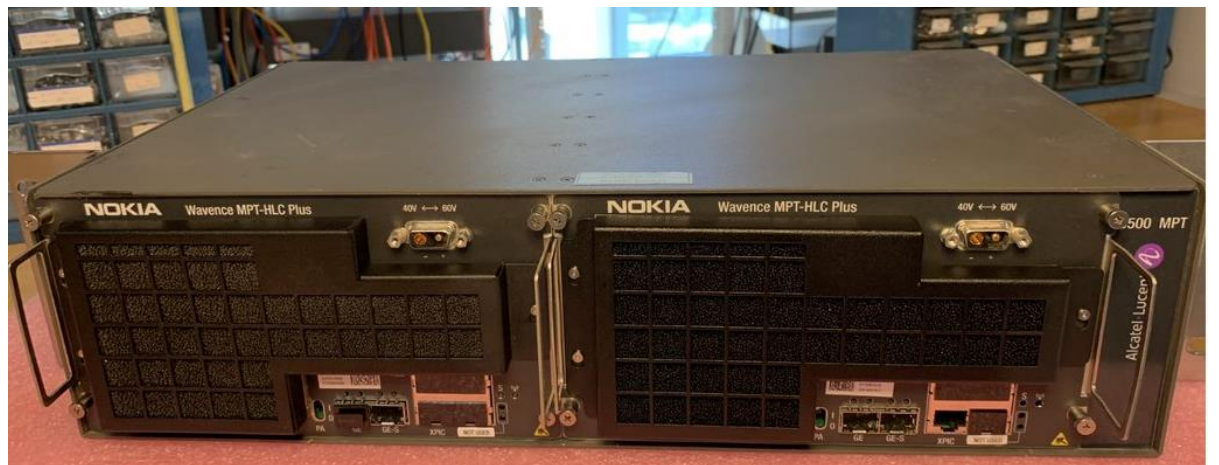
Figure 4: Front of the chassis with two MPT-HLC modules inserted
