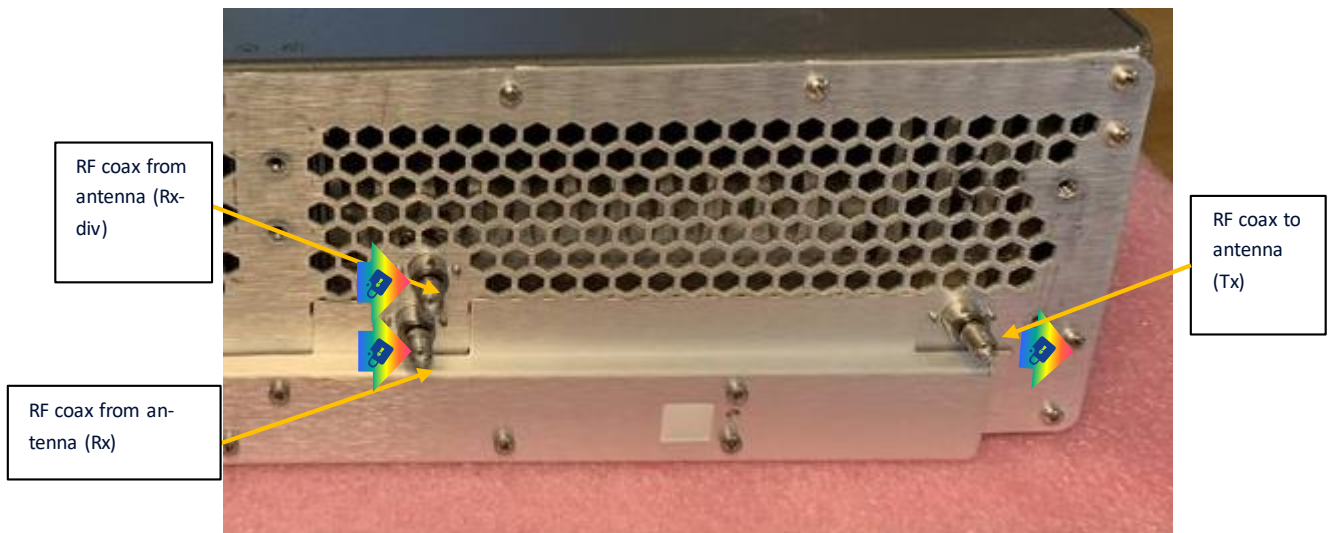
Figure 7: MPT-HLC ports and interfaces on Backplane
