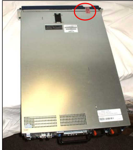
Figure 3 - Tamper-Evident Label Application Instruction at the Front
