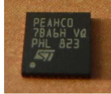
Figure 8: Picture of the Cryptographic Module (VQFN32) – Marking PEAHC0
