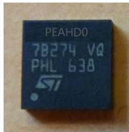
Figure 12: Picture of the Cryptographic Module (VQFN32) – Marking PEAHD0
