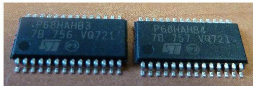
Figure 3: Picture of the Cryptographic Module (TSSOP28) – Marking P68HAHB3 & P68HAHB4
