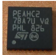
Figure 10: Picture of the Cryptographic Module (VQFN32) – Marking PEAHC2
