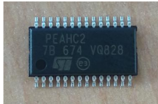
Figure 10: Picture of the Cryptographic Module (VQFN32) – Marking PEAHC2
