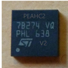
Figure 14: Picture of the Cryptographic Module (VQFN32) – Marking PEAHC2 V2
