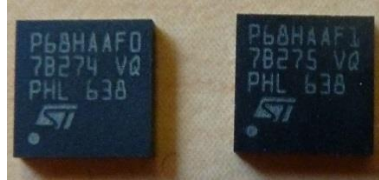
Figure 2: Picture of the Cryptographic Module (VQFN32) – Marking P68HAAF0 / P68HAAF1
